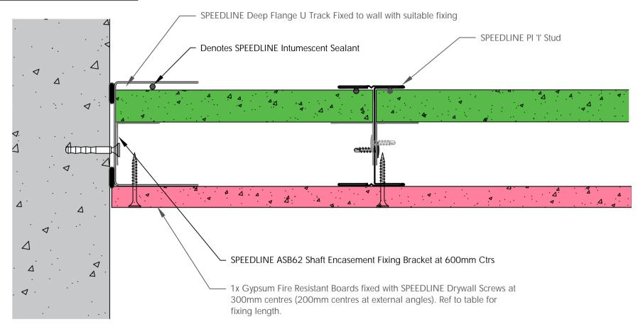
DATE: 30/04/18 CDR No: 1096 SCALE: NTS SHAFT ENCASEMENT PARTITION SYSTEM - START WALL
