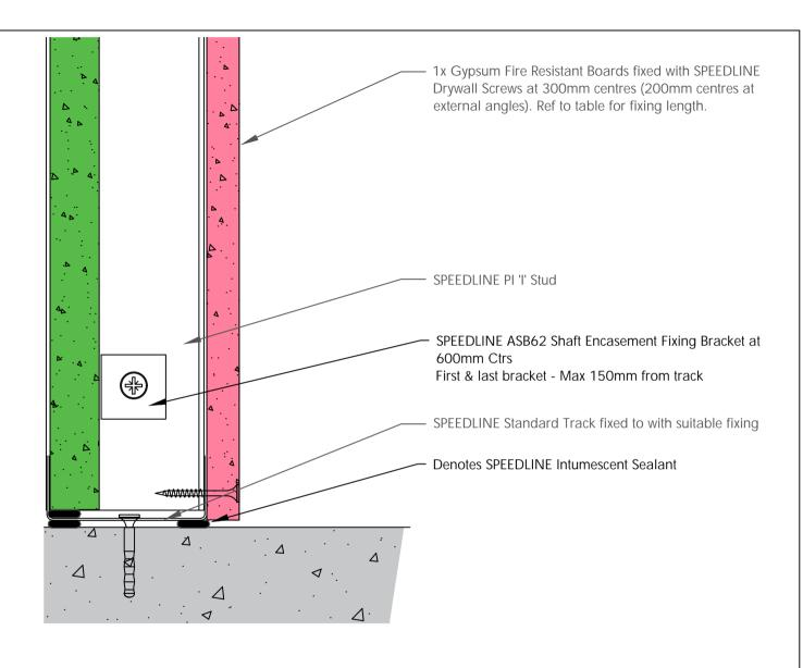
CDR No: 1090 SCALE: NTS DATE: 30/04/18 SHAFT ENCASEMENT PARTITION SYSTEM - BASE DETAIL
